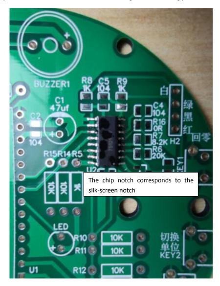
2: Find the metal film resistor and the plug-in transistor, and weld them at the corresponding positions. The resistance should match the resistance value on the silk screen; (welding sequence: from short to high, from small to large)
